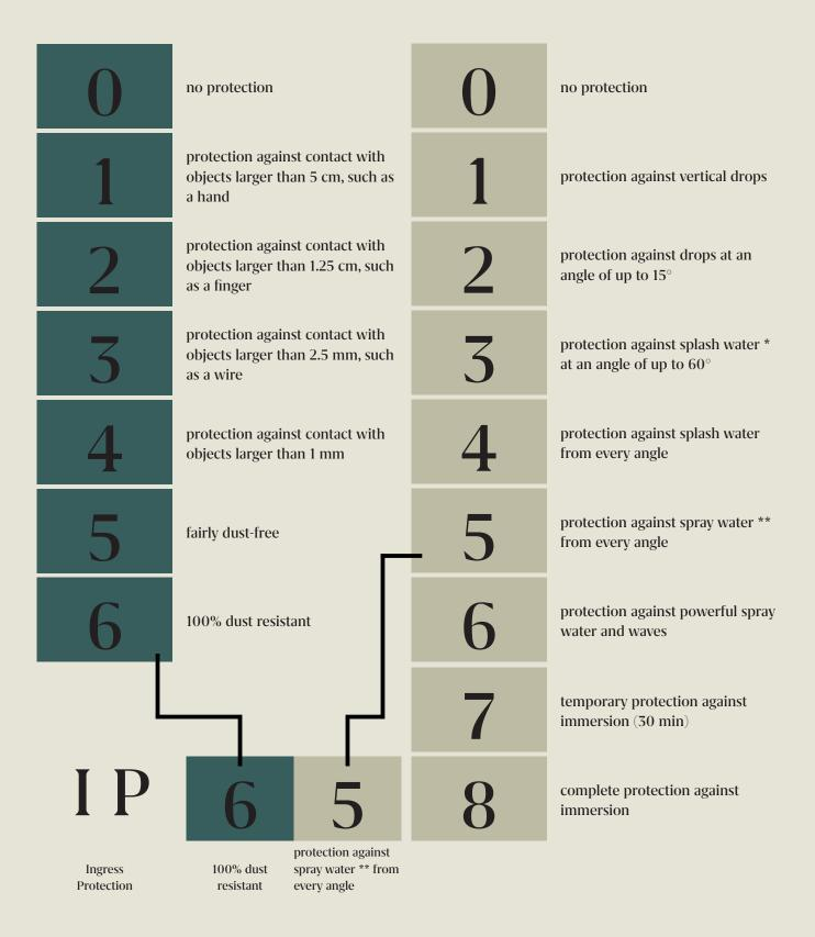
\* splash water = protected against splashing water, for example rain
