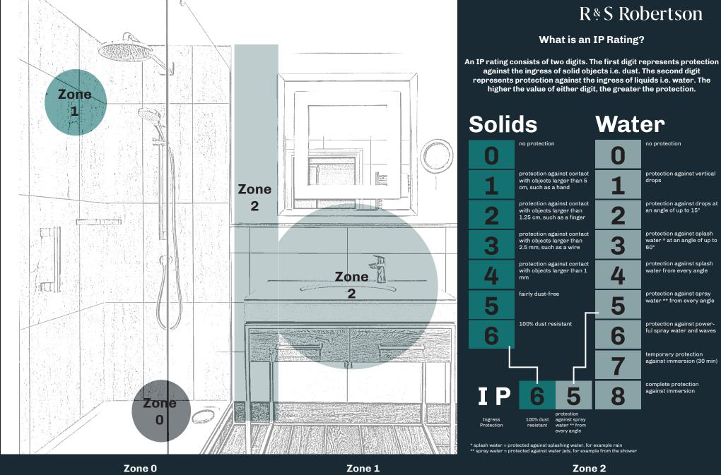
Minimum IP67 Minimum IP45 Minimum IP44
